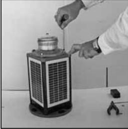
1. Remove 4 x M6 x 20 socket head cap screws (SHCS) and 4 x M6 nylon washers and disconnect the light head from the chassis
