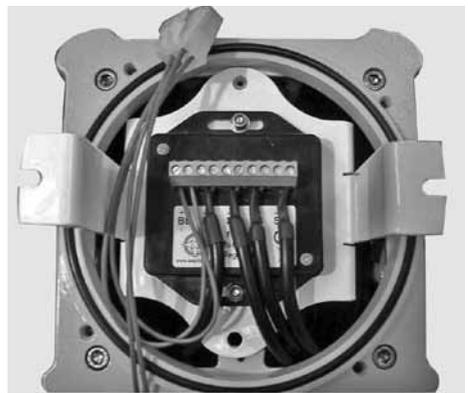
SL10 AMP Regulator shown when correctly fitted
