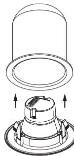
Slide the LED downlight up into the recessed housing with the ceiling.
