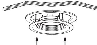
Push the LED retrofit trim into the recessed light fixture. Continue to push the LED trim until its outer edge is flush with the ceiling surface.
