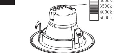
Before installation, select your preferred CCT by moving the switch to either 2700K, 3000K, 3500K, 4000K or 5000K.
