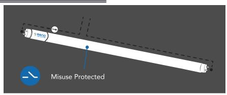
Misuse - Protected function ,if forgot to by-pass the ballast, the lamp won't work, no risk of fire or cap melting.
