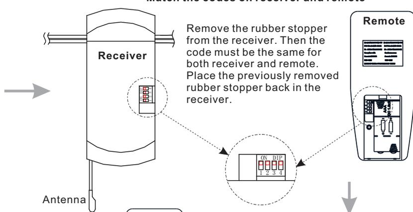
Remove the rubber stopper from the receiver. Then the code must be the same for both receiver and remote. Place the previously removed rubber stopper back in the receiver.
