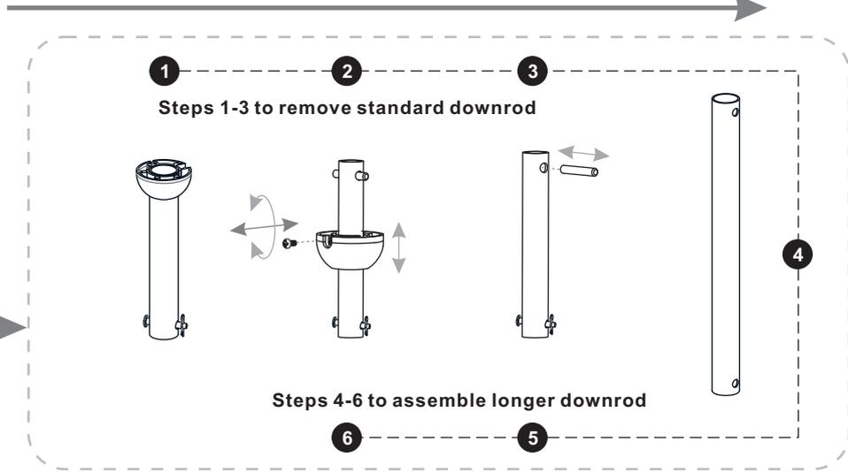
**3 Install Rod to Fixture Body**
