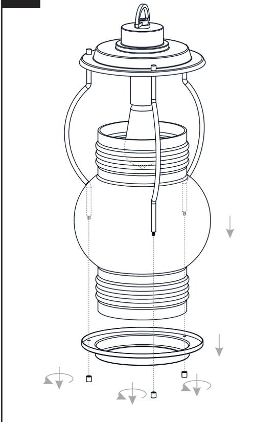
Reverse above steps to reinstall the replacement Glass panels onto fixture.
