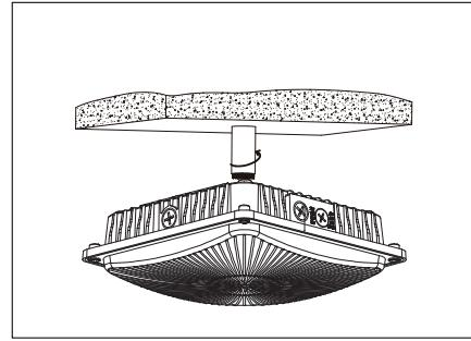
3. Screw the pole into the hole on top of Canopy fixture. Installation done.
