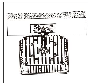
4. Slide the Canopy fixture into bracket, and secure the screw on side of the fixture to prevent the fixture slide out from the bracket. Installation done.
