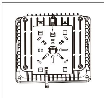
2. Install the bracket on J-box, and put the wire through the central hole for wiring.
