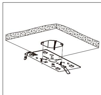
3. Attach the Canopy fixture with bracket by putting the ring on clips again. Connect the Black wire for Line, White for Neutral, Yellow/Green for Ground. See wiring diagram for details
