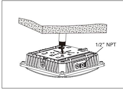
2. Connect the wire from pole with Canopy, Black wire for Line, White for Neutral, Yellow Green for Ground. See wiring diagram for details
