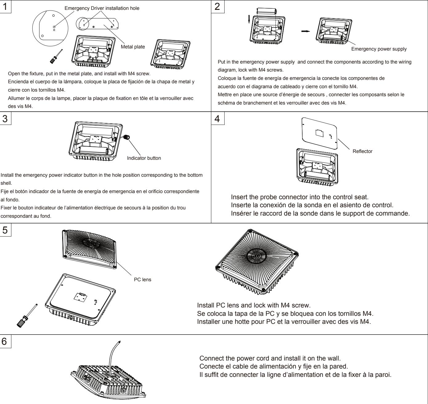
\*Use silicone sealant around plate and all opening to ensure a weather proof seal.
