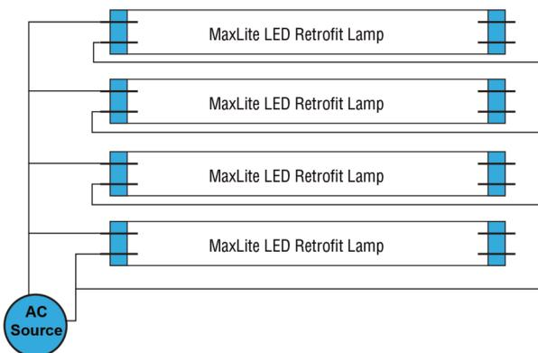
**Note: These fixtures are for use only with lamps wired per the above example. Serious risk of electrocution, or fire if non-compatible lamp is installed.**
