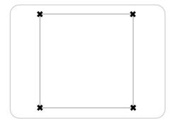
Locate secure structural member and inspect for damage. Mount top surface mount bracket onto flat surface with 4 x #10 screws. Use drill pattern figure above.
