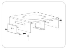
Lift LED high bay and guide Z brackets through top bracket slot openings and let rest. Secure Z brackets to surface mount bracket using 2 x #8 screws.
