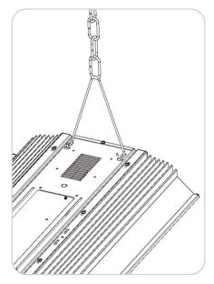
Run chains through V hooks and attach onto fixture.
