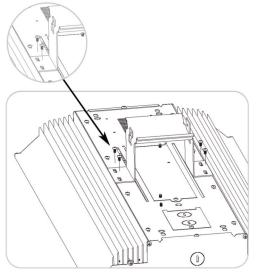
Attach base bracket onto fixture by inserting 4 x #8 screws
