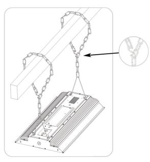
Locate secure structural member and inspect for damage. Secure chains around member and lock with S hook.
