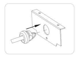
Locate secure threaded pole and inspect for damage. Use the cord grip provided to securely attach wires onto side bracket.
