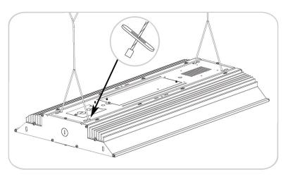
Adjust fixture height by drawing cable through gripper.
