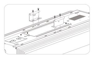
Secure 2 Z brackets onto fixture with 4 x #8 screws. Follow figure 3 for proper installation guidelines for methods of positioning the Z bracket.
