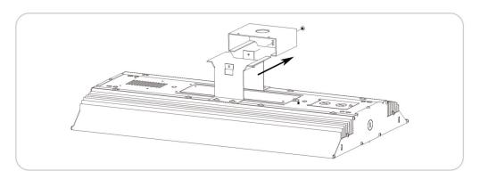
Slide assembled fixture onto pole. Wire input wires to fixture.
