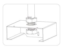
Secure top pendant mount bracket onto stem/pole by placing one nut before installing bracket and one nut after.
