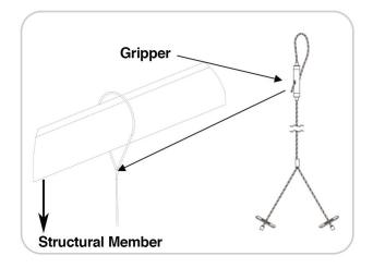
Locate secure structural member and inspect for damage. Secure aircraft cable around member and run through gripper to fasten. Cable enters and exits through side of gripper.
