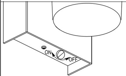
If the fixture doesn't light, check switch on fixture to make sure it is turned on.
