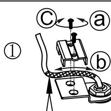
Always keep the fiberglass sleeving between the metal strain relief and the cord to protect the cord from damage
