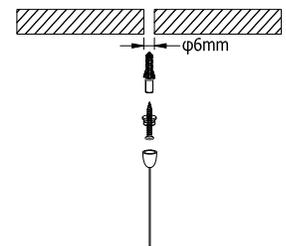
6. The mounting length from ceiling can then be altered by adjusting the wire rope with the steel wire buckle and wire rope fastening screw. (spare part #5 and #4)
