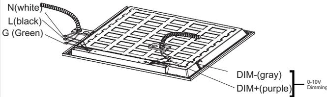
4. Replace the driver cover and secure with screws.
