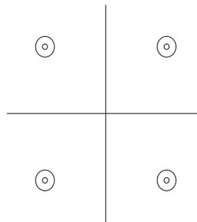
4. For each hole location, drill the expansion pipe (spare part #10 on diagram) firstly into the newly formed insert, and fasten securely with suspension fixed bushings and self-tapping M4 screws (spare part #9 and #8 respectively)
