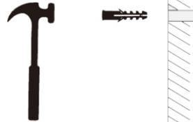
3. Use a hammer to hammer the nylon expansion anchors into the drilled holes on the wall.
