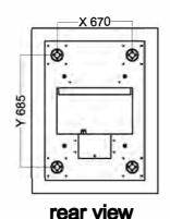
1) Measure the Distance between the holes on the back of the mirror, then proceed to mark the wall to match. Ensure that the markings are aligned with the studs in the
