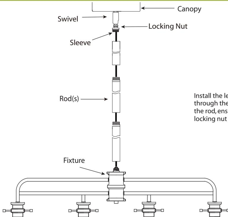
Install the length of rod that is required by threading wire through the rod and screwing it to the fixture. Install swivel to the rod, ensuring that the sleeve is at the swivel. Tighten the locking nut to secure rod to the fixture.
