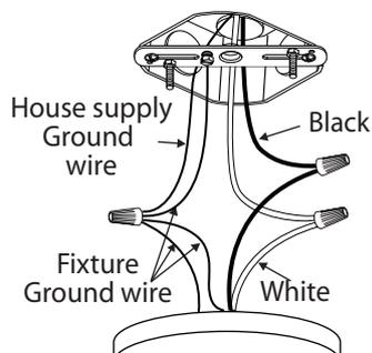
Connect the ground wires (bare copper or green) from your fixture to the ground wire (bare copper or green) or ground screw in the electrical outlet box. Attach the black wire from the light fixture to the black wire in the electrical box. Attach the white wire from the light fixture to the white wire in the electrical box.
