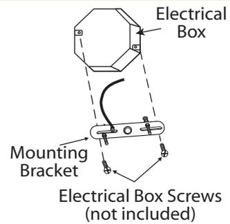
Mount the mounting bracket to electrical box using electrical box screws (not included). Make sure the studs on the mounting bracket are facing out from the electrical box.
