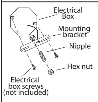
3. Loosen the upper connector from nipple. Attach the mounting bracket to the electrical box using electrical box screws (not included). Attach the nipple to the mounting bracket and adjust until it will clear the canopy when assembled (Place the canopy over the nipple and tighten the upper connector onto the nipple until snug. The upper connector should hold the canopy snug to the ceiling). Lock the nipple in the correct position using the hex nut.
