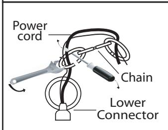
4. To attach chain loop to light fixture, use a screwdriver and wrench to open and close chain loop. Ensure to close the opening. Weave the power cord and ground wire through the links in the chain.
