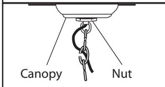
8. Slide the canopy up the chain and over the upper connector. Slide the nut up the chain and thread onto the upper connector.
