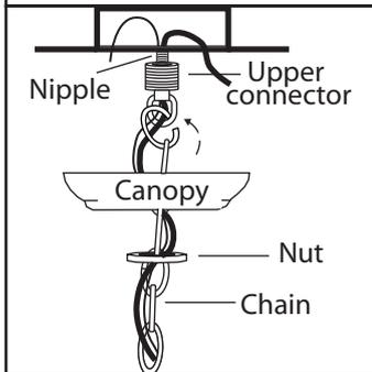
5. Loosen the nut on the upper connector and slide it down the chain towards the lower connector. Slide the canopy down the chain towards the lower connector. Feed the wire through nut, canopy, the upper connector and onto the nipple. Tighten the upper connector onto the nipple. Spread the other end of the chain open and fasten to the upper connector. Ensure the opening is closed.
