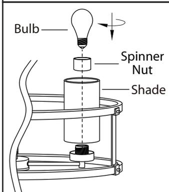
9. Remove spinner nut from socket. Position shade on lamp and secure with spinner nut.
