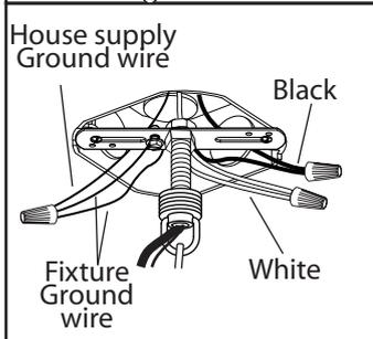
6. Connect the ground wires (bare copper or green) from your fixture to the ground wire (bare copper or green) or ground screw in the electrical box. Connect the black wire (or wire marked "SPT-1") from the fixture to the black wire in the electrical box and connect the white wire (or the wire with ribbed side) from the fixture to the white wire in the electrical box.
